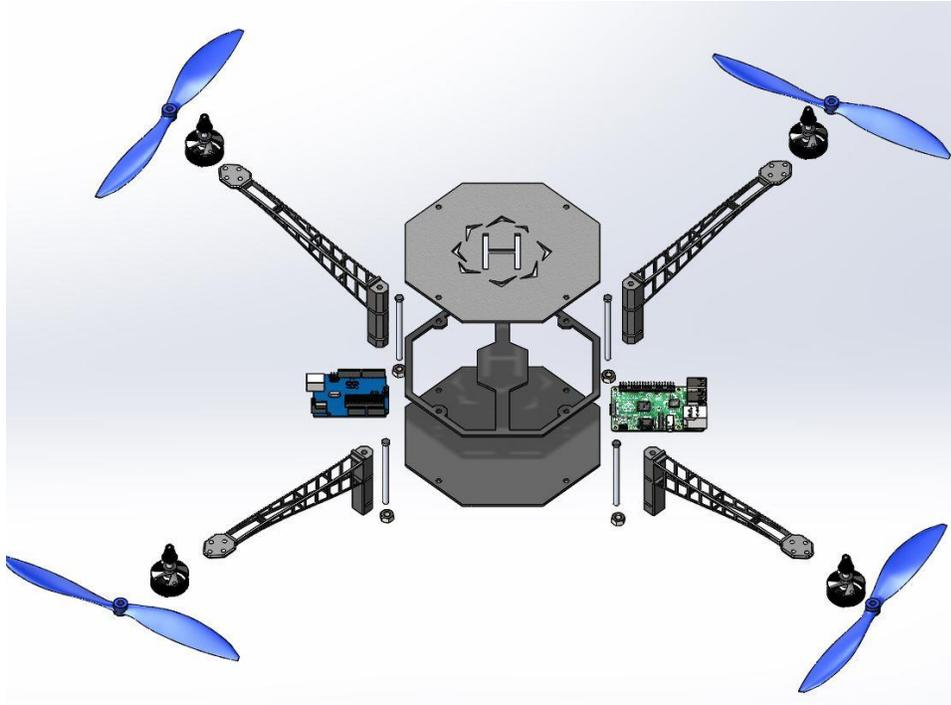
This is an exploded view of the current iteration of the final design. This illustrates the mounting capabilities of the middle plate and the construction of the arms.
