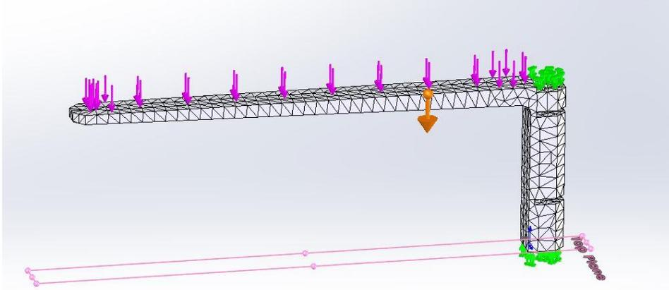
This picture shows the setup of the test. Green arrows show where the object will be fixed (in this case it would be to the chassis). Pink arrows are forces from the motor and propeller generating thrust. The orange arrow is the force from the arms own mass. The black lines patterned around the arm is the mesh. Because this was a simple test, the mesh is relatively rough, meaning the test is less accurate.
