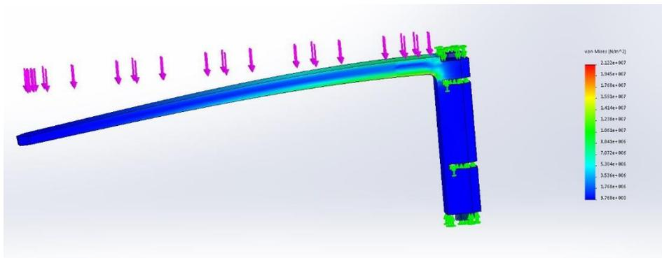
I tested the new arm design with what is the expected force from its own mass, the mass of the motor, and the force produced by the propeller generating thrust. This arm is made of ABS, so it is not entirely accurate.
