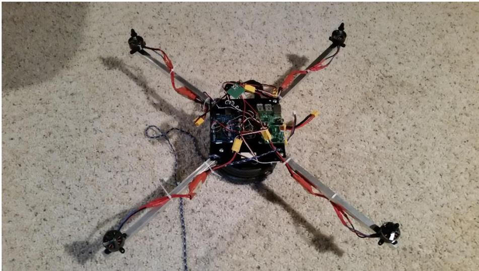
The chassis weighs approximately 1600 grams, which is relatively lighter than the expected 2000 grams from the initial project proposal. One small, but major, improvement was adding a switch, which can be seen on the right side of the quad (black box). Before I added the switch, the only way to power on and off the quadcopter was disconnecting the battery.
