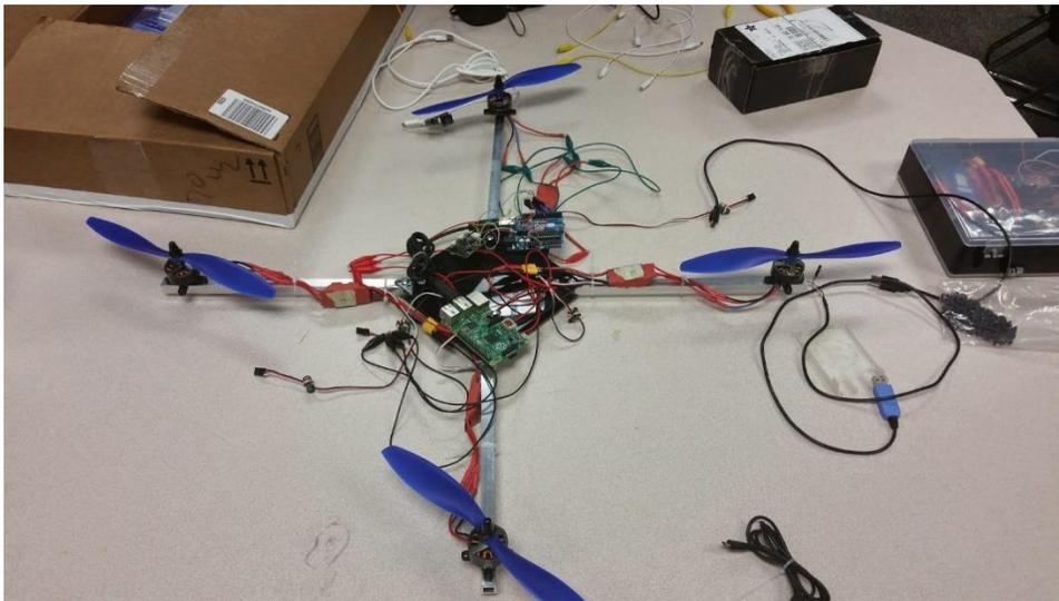
Once the electronics were mounted, including the battery, the quadcopter was attached to a weighted base for testing after the electronics were stably mounted.
